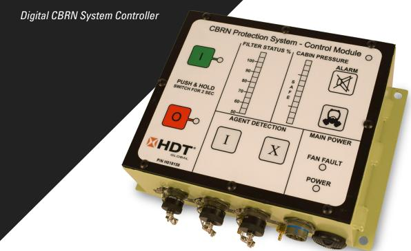
The Universal System Control Module (USCM) is a digital system controller that monitors the protected volume (Toxic Free Area – TFA) pressure relative to the outside ambient pressure and provides variable-speed signals to the filtration system fan controller to maintain constant pressure in the TFA.
