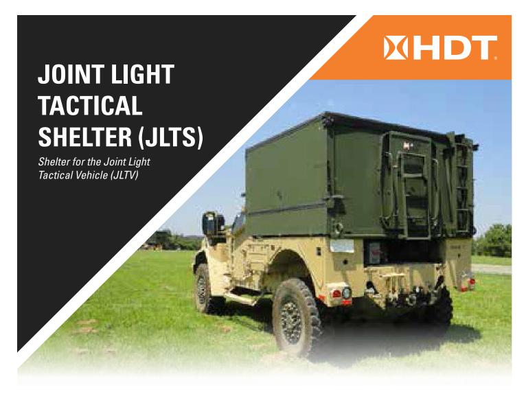
A force multiplier for the Joint Light Tactical Vehicle (JLTV), the Joint Light Tactical Shelter (JLTS) is a state-of-the-art mobile shelter solution for the JLTV. Engineered for durability and operational efficiency, the JLTS features lightweight, robust composite walls and an innovative roof system that can be extended up to create a spacious interior for up to five personnel to comfortably stand and operate.
