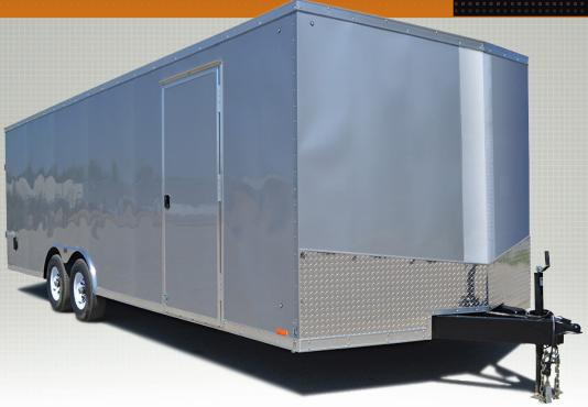
The HDT Enclosed Cargo Trailer is a commercial-grade enclosed trailer capable of hauling over 3,300 pounds of cargo. This rugged trailer features tube main frame construction, ¾" high-performance floor with 5,000 lb recessed bolted D-rings, white vinyl walls and ceiling. A ramp rear door with spring assist and a 36" side door with flushlock and metal holdbacks make the trailer easy to load and unload and a one-piece aluminum roof means that your gear stays dry.
