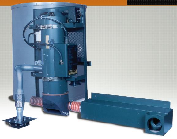
HDT's Cargo Bay Heater Kit (CBHK) allows for installation of an auxiliary heating system in the cargo area of van bodies and larger heavy-wheeled vehicles. Once installed, this system provides up to 60,000 BTU/H (17.5 kW) of warm air in the cargo area and battery compartment. The CBHK incorporates the HDT A20 Heater, a compact multi-fuel unit that was originally developed for the United States Army Tank-Automotive Armaments Command (TACOM).
